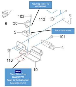
Bottom view of the cut carriage assembly. Note the position of the filter sheet.
