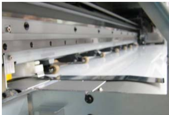
New pinch roller & media guide design
