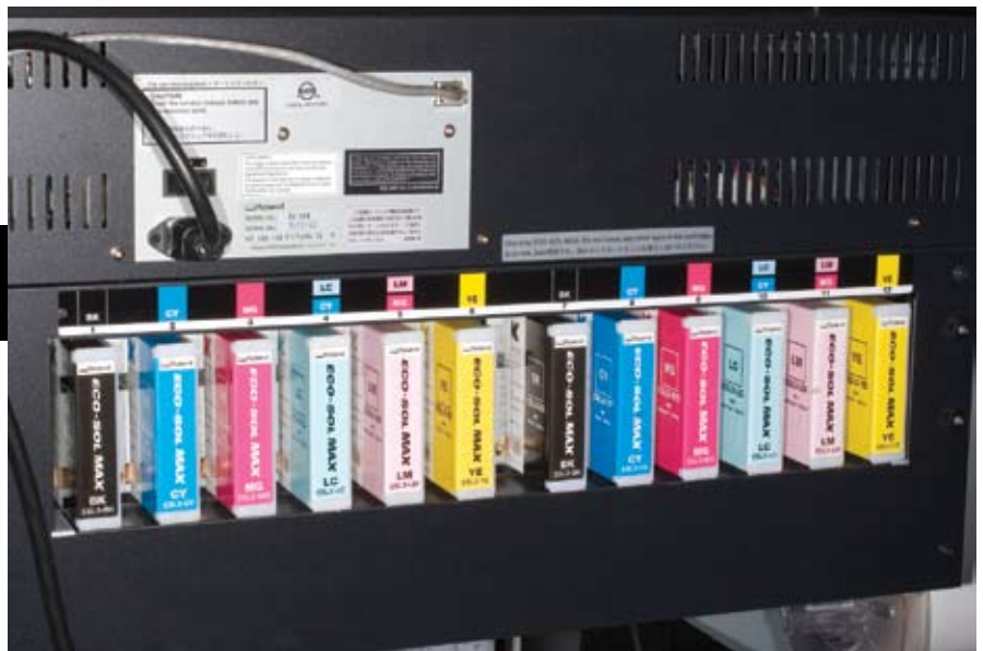
Fig. 3. For faster, higher-quality prints, Roland doubled the XC-540's ink set.
