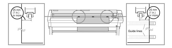
4 While keeping the material stretched taut, raise the sheet loading lever to secure the material in place. When using a material which is narrower than 762 mm (30 in.), do not lower the middle pinch roller.
