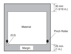
The origin point is set at the location where the material is loaded, near the left pinch roller.
