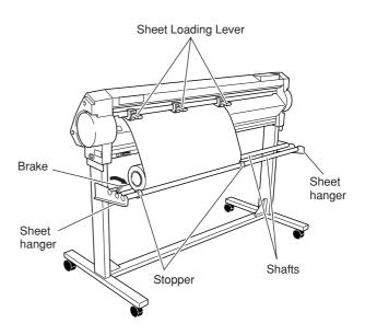
Performing high-speed cutting when only a little roll material remains may cause the roll to fall off the shaft. If this happens, it may help to pass the shaft through the roll.
