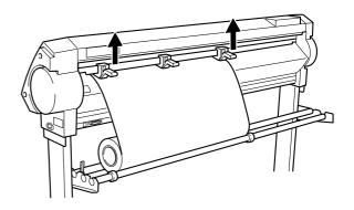
Position the stoppers so that they lightly touch the edges of the roll, and secure in place by tightening the screws.
