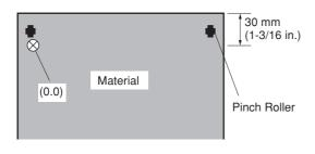
Set the origin point at a location having a margin of 30 mm from the trailing edge of the material. When in this state, the cutting area is zero.
