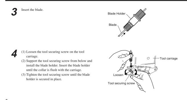
When you're using general sign material, use with the cap tightened all the way to the top (maximum amount of blade extension: 2.5 mm). When cutting material whose carrier paper is thin with respect to the adhesive layer (that is, the material thickness), or when performing half-cutting for material with no carrier paper, adjust the blade tip so that the tip does not pierce the carrier paper. For more information, see "5-1 Detailed Cutting-condition Settings."
