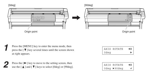
Press the [ENTER] key to enable the coordinates.Press the [] key to exit the menu mode.
