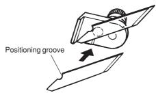
The knife is secured in place by the magnet.
