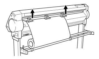
Position the stoppers so that they lightly touch the edges of the roll and secure in place by tightening the screws so that the rolled material does not move from side to side during material feed.
