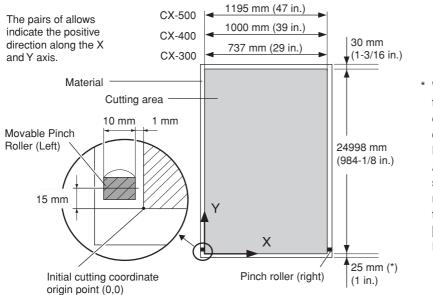
When you select [F-EDGE] or [PIECE], this is 25 mm. When you select [ROLL], everything toward the front from the origin point is the margin. (See "The Location of the Origin Point Immediately After Loading Material" elsewhere in this section.) When you have separated the material using the [SHEET CUT] key, this is the value set for [MARGIN] at the [AUTOCUT MENU]. Refer to "7-3 List of Functions."
