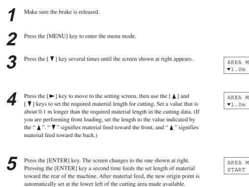
Press the [ ] key to exit the menu mode. If the material is crooked and looks like it might come loose from the pinch rollers, or actually does come loose, please reload the material.
