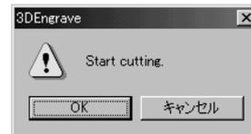
If you carried out draft cutting, then go back to "Generating the Tool Path" on page 36 and perform finishing. Be sure not to remove the material at this time.
