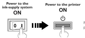
First switch on the power to the system, and then switch on the printer.
