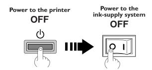
First switch off the power to the printer, and then switch off the system.
