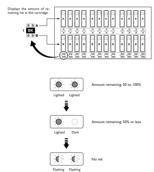
The display shows an approximate guide to the amount of remaining ink, which may differ somewhat from the actual amount remaining. Also, the displayed information may differ greatly from the actual amount remaining if you insert a partly used ink cartridge or change cartridges while the power is off.
