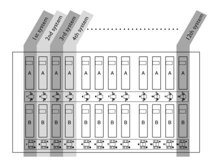
Ink is not depleted evenly from the A and B cartridges. This is done to prevent the two cartridges from becoming empty at the same time.
