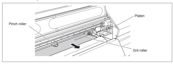
3 Make sure both edges of the media are above the grit rollers, then place pinch rollers over all grit rollers covered by the media.
