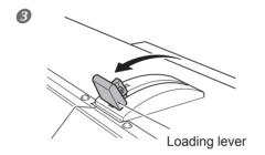
Pull back the loading lever. The media is secured in place.
