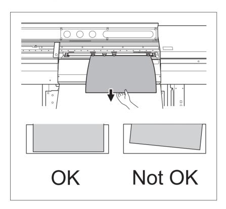
2 Pull back the loading lever. The media is secured in place.
