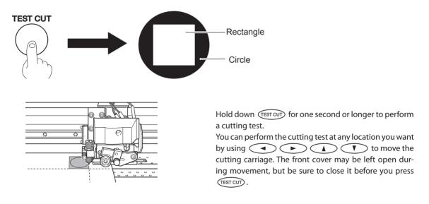
Peel off the cut shapes to verify the cutting quality, and make the setting for blade force. If two shapes peel off together, make the setting for blade force.
