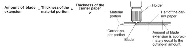
Note that making the amount of blade extension too small may cause the end of the cap for the blade holder to touch and damage the printed surface. It's important to be especially careful about this when you're using media that has poor ink-adhesion properties.
