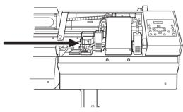
5. Insert the head-unit tool into the hole at the bottom of the machine and turn gently. The cap unit rises.
