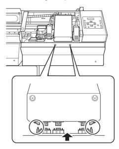
7. When the heads make contact with the cap unit, turn the tool one or two turns more.
