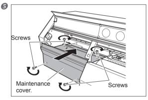
Open the front cover and attach the maintenance cover.
