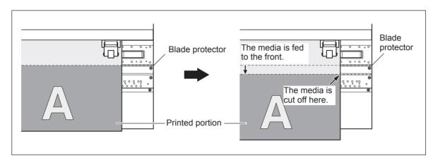
You can make the setting in the software RIP for automatic media cutoff after printing or cutting has finished. For information on how to make the setting, refer to the documentation for the software RIP you're using.
