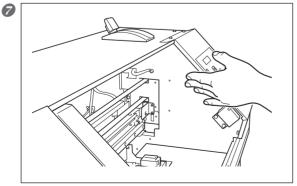
Touch the location shown in the figure to discharge any static electricity.
