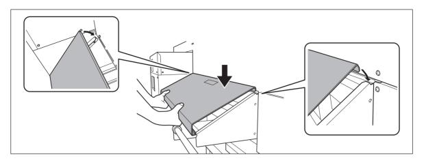
Pass the leading edge of the media between the grit rollers and the pinch rollers, and feed it out as far as the platen.
