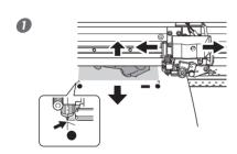
Use to align the center of the blade with the location shown in the figure.
