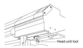
6. Make the guides at the edges of the print heads line up with the guides at the edges of the cap unit. Turn the tool further to bring the cap unit near the heads.
