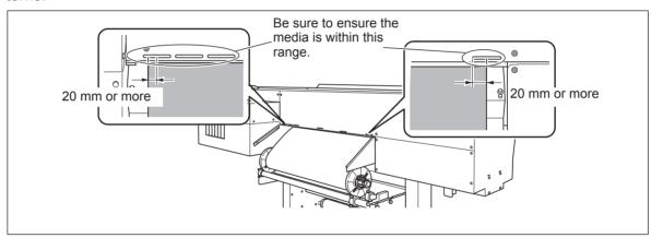
Secure the stoppers in place in alignment with the width of the media.
