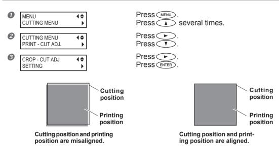
When adjustment is needed, go on to the steps below.
