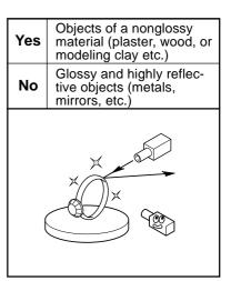
In such cases, applying a surface coat (primer coat) to the object may make scanning possible.
