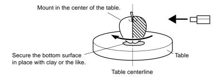
The table rotates during scanning. Using double-sided tape, clay, or the like, fasten the object in place securely so that it will not fall over or slip. Any slipping of the object makes correct scanning impossible.
