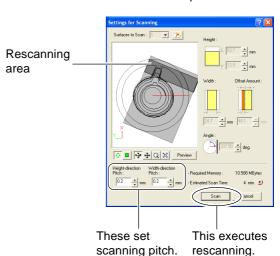
You can perform rescanning as many times as you like after basic scanning. Also, when you want to redo scanning after checking the scanning results, you can go back to the previous state before rescanning by clicking the [ ] button. For detailed information on rescanning methods, refer to the online help for Dr. PICZA3.
