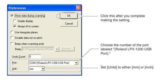
This completes all the preparations you need to make to perform scanning using the machine.
