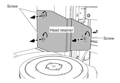
Never touch or try to move and internal equipment other than the head retainer and the screws.
