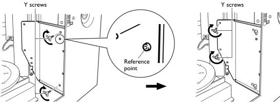
Using the protrusion at the front of the machine as the reference point, provisionally tighten at the front.
