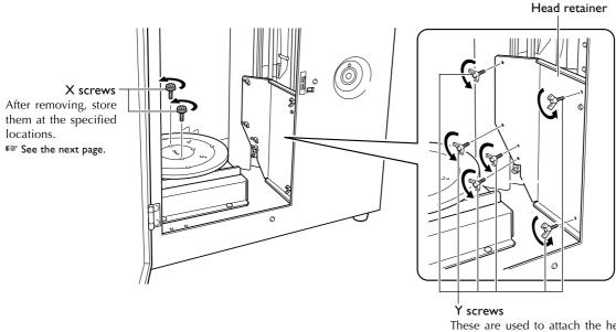
These are used to attach the head retainer and the included AC adapter holder at the back of the machine.
