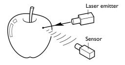
It performs scanning as it rotates the scan object and moves the laser beam from bottom to top.
