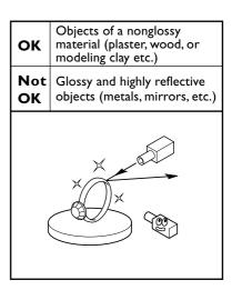
In such cases, applying a surface coat (primer coat) to the object may make scanning possible. Note: Avoid highly reflective objects because of danger of eye injury.
