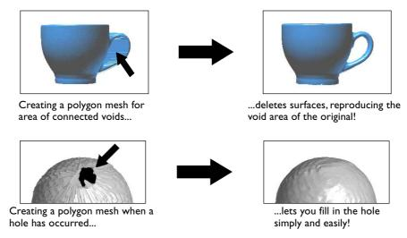
A polygon mesh is composed of polygons created by estimating the original shape of the scan object from the scanning points. They differ from the polygons displayed immediately after scanning, which are generated simply by connecting the scanning points.
