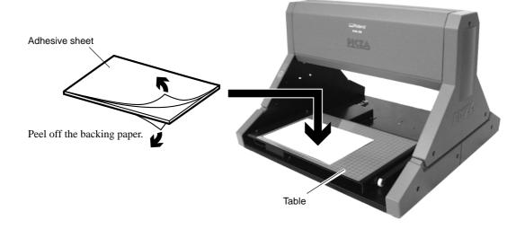
**2** Place the scan object on the adhesive sheet, and gently press it down to secure it in place.
