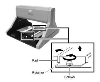
Before using the unit, remove the screws and the retainer shown in the figure.
