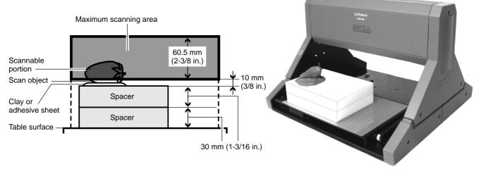
3) Use clay or on adhesive sheet to secure the scan object in place.
