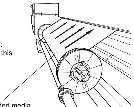
If there is slackness in the loaded media, the media may move at an angle and come loose from the pinch rollers.
