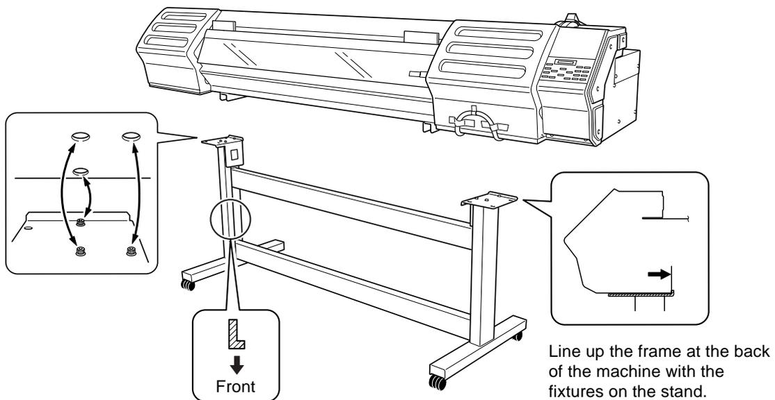
Line up the frame at the back of the machine with the fixtures on the stand.
