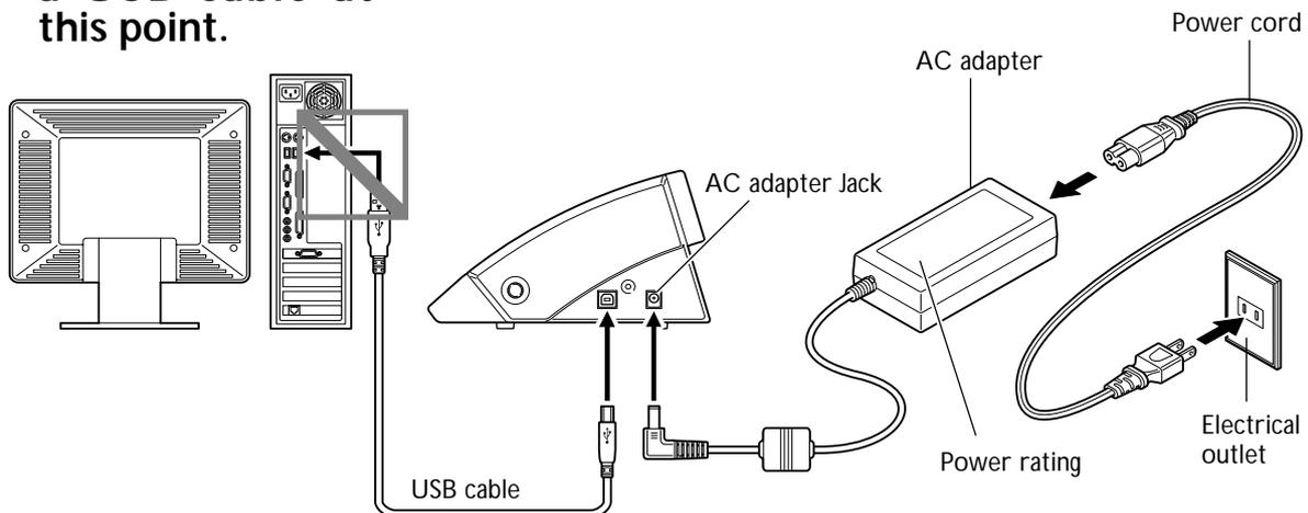
You make the connection to the computer using the included USB cable. Connect the USB cable at the time indicated in the driver installation procedures. Driver installation may fail and the machine may become unusable if you connect a USB cable before starting installing the driver.
