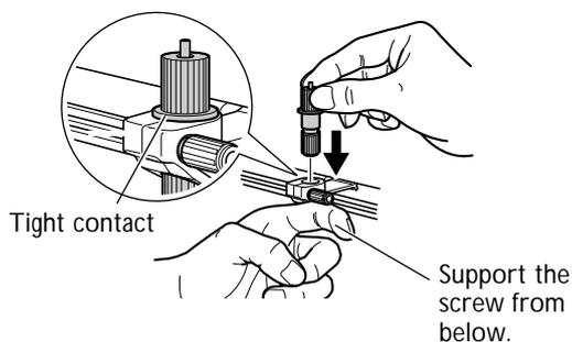
Support the screw from below and insert the blade holder.
