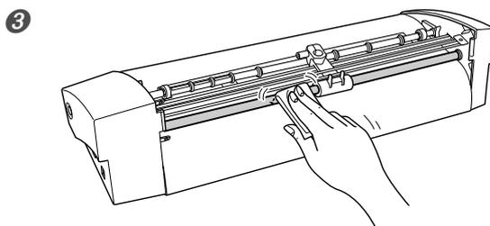
Wipe and remove dust adhering to the shaft.
