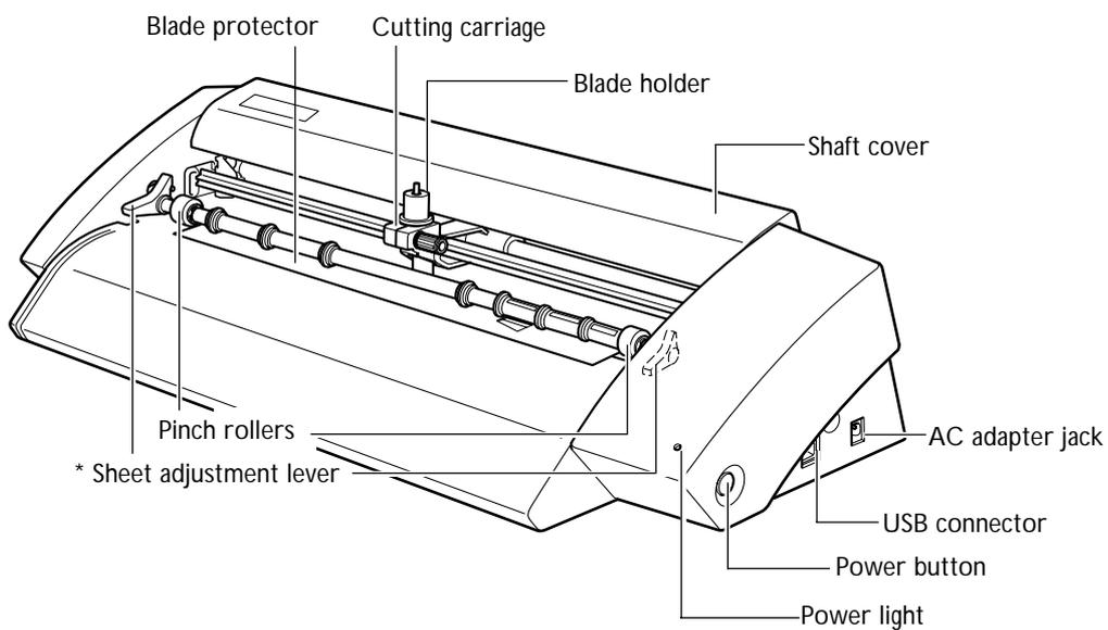
\* The SV-15 has sheet adjustment levers on the left and right. The SV-12/8 has a sheet adjustment lever only on the right.
