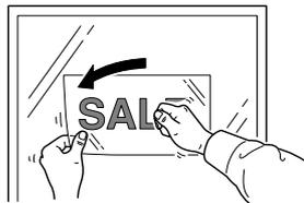
Affix the material together with the joined application tape to the target object, then press down on it from above.
