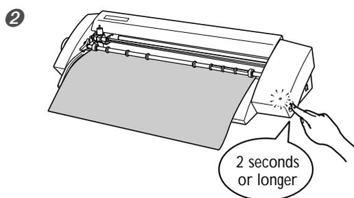
With the power light on, hold down the power button for 2 seconds or longer.
