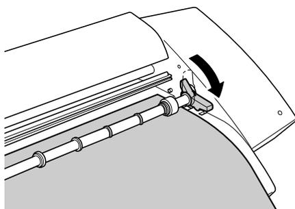
Lower the sheet adjustment lever to fix the material in place.
