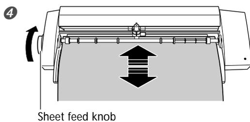
Turn the sheet feed knob and move the material into the machine and then back out. Verify that the material does not come loose.
