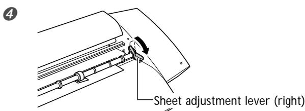
Lower the sheet adjustment lever on the right side.
