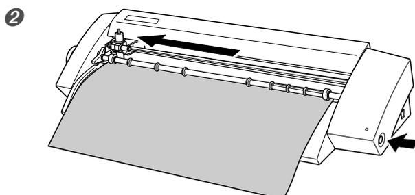
Press the power button again and turn the machine on.
