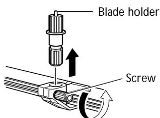
Loosen the screw, remove the blade holder.
