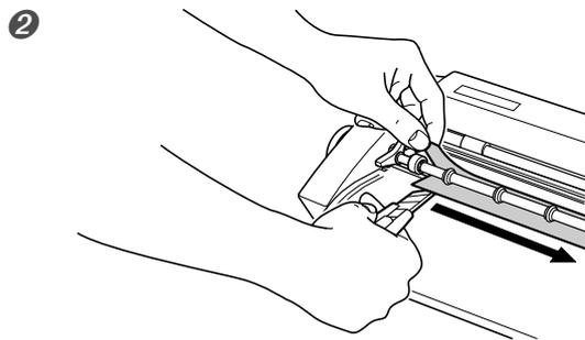
Peel the blade protector from the main unit. Use a commercially available retractable knife to facilitate removal. If you are using the SV-15, raise the left/right sheet adjustment levers and remove the blade protector.
