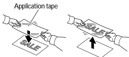
Cut the application tape to the required size. Cover the cut material flush with the application tape to prevent any air from getting underneath, then transfer the material.
