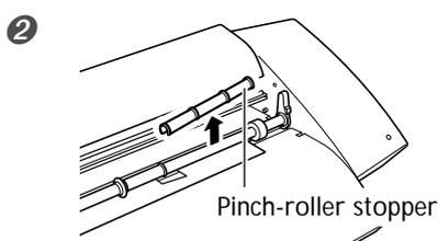
Remove the pinch-roller stopper. Do not use excessive force to widen the opening when removing the pinch-roller stopper. If the opening is widened, the stopper may become loose and fall out when it is next attached to the unit.
