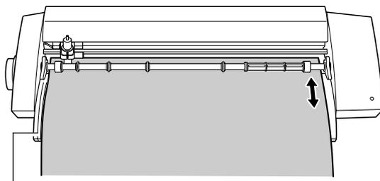
Move the material backward and forward and align the left edge of the material with the guide line.
