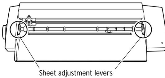
For the SV-15, lower the left/right sheet adjustment levers.
