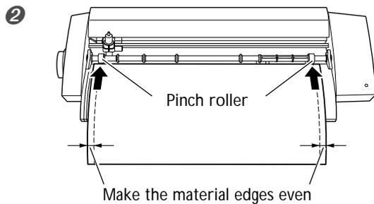
Verify that the material is narrow enough to be loaded and that it touches the pinch rollers.
