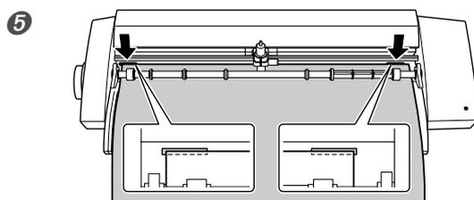
Align the material edge with the marks at the back of the blade protector.
