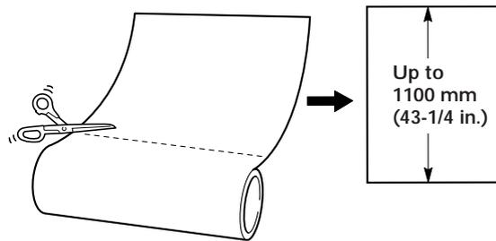
> Cut the material at a right angle. If the front edge of the material is uneven, it may feed improperly during cutting and could skew diagonally and come loose.
