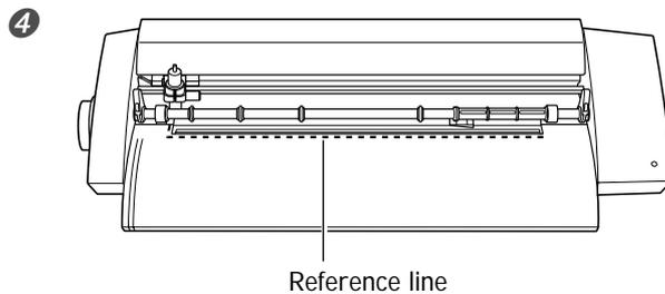
Place the replacement blade protector into the machine. Align the blade protector using the reference line displayed on the machine.
