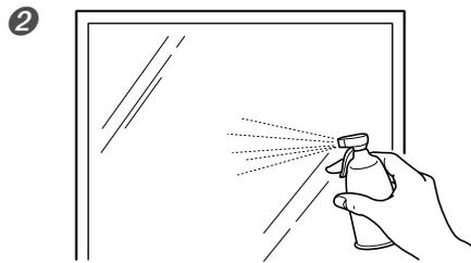
Remove any dust and grease from the application surface.
