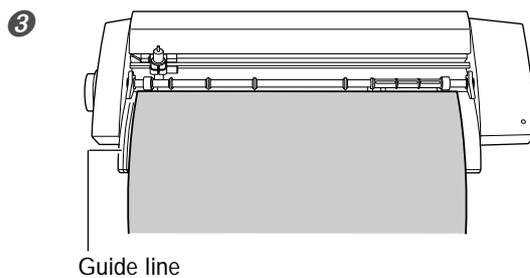
Verify that the left edge of the material is parallel with the guide line.
