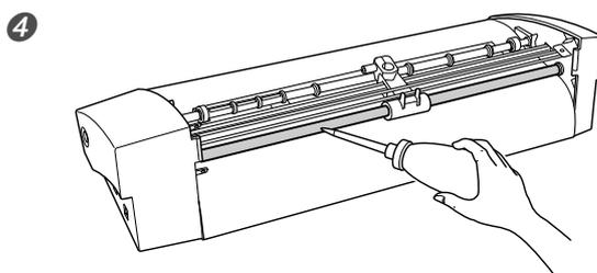
Use machine oil to lightly lubricate the shaft section indicated in the figure to the left.
