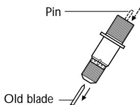
Press the pin and remove the old blade. Press in until you can no longer see the pin.
