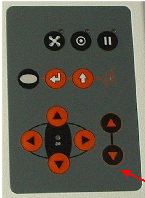
Figure 21: height adjustment via Z positioning keys
