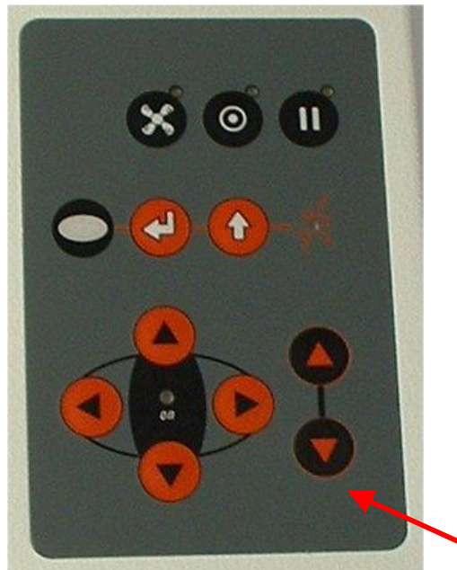
height adjustment via Z positioning keys
