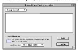
4 Accept the default selection of Easy Install and specify the location to which to install the software. Click Install when you are finished. A status window displays the progress of the installation.
