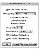
By checking Enable Driver Options, printer-specific options defined here are sent to your printer to override option settings currently made through your printer menu. When it's unchecked, the printer settings are used.
