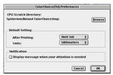
CPSI Scratch Directory—This is the location used to store information during processing. If you have multiple drives, you can use the Browse button to relocate the Scratch Directory to the drive with the most storage space. Doing this will allow you to process larger files without generating memory errors.
