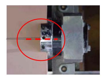
NOTE: If the center of either chucking cannot fit to the center of workpiece, the workpiece might turn eccentricity.
