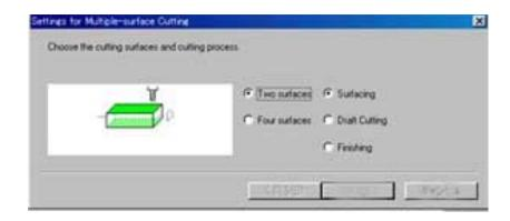
Note: You cannot skip the process of Surfacing. Please carry out in order 1. Surfacing, 2, Draft, 3. Finishing.
