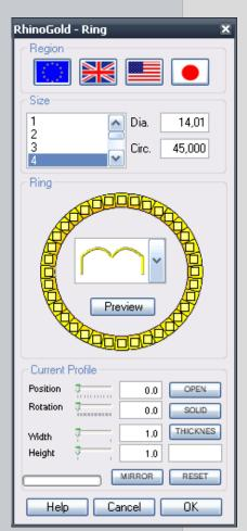
Wizard for creating rings according to profiles. It is very quick and practical for new users. We choose the size and place the profiles in position in the ring's side view.
