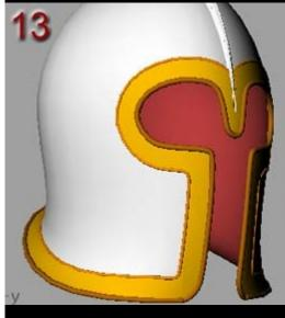
Each pipe and decorative trim surface have now been put on separate layers with different OpenGL Render colours to check for proper overlap with no gaps. If necessary pull control points to fix any problems.
