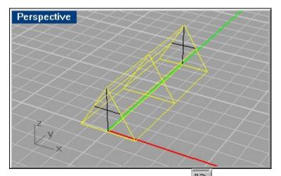
STEP 3: Before continuing, go to the right view, select the rotation tool; place the mouse at the center of the object and click once. Rhino will ask for the amount of degrees, type in 90. The object will rotate by 90° in all views.
