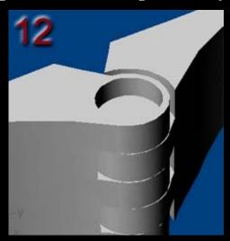
Step 12 - Create an additional cylinder slightly smaller in diameter than the cylinders you just used. Use this to boolean difference out a depression in the top pf the hinge.
