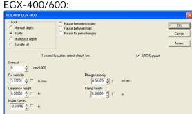
10. Once set, highlight the Braille only and click on Engrave and Output. The engrave window should only show the Braille drill and at this point click the engrave icon to output the file. Ensure that you have the proper tool installed (0.060" Parallel or 0.060" Replaceable drill cutter) and that your XY & Z settings are set accordingly.
